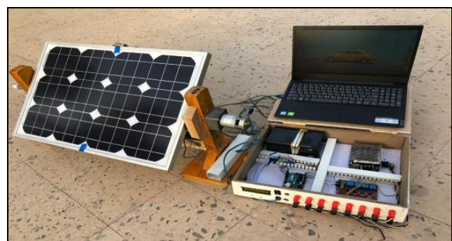
Fig.18 Overall solar tracking experimental set-up
