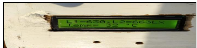
Fig.12 LCD shows the temperature and LDR1, 2 values
