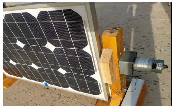
Fig.13 DC motor and tracking system experimental set-up
