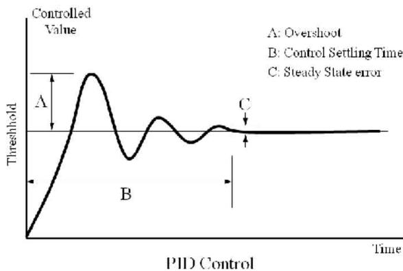
Figure (2): Flow rate response with PID controller
