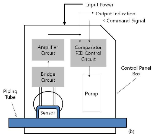
Figure (3): Flow rate controller : (a) photograph of control panel box, (b) operational diagram
