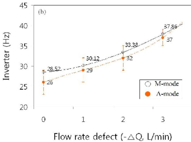
Figure (6): Variations of pump control frequency according to flow rate defect : (a) water, (b) corn oil
