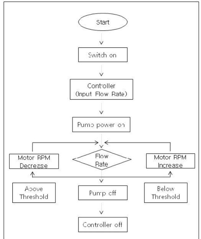
Figure (4): Basic logic diagram for constant flow rate control
