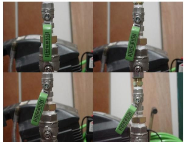
Figure (5): Flow control valve for hydraulic pumping head loss
