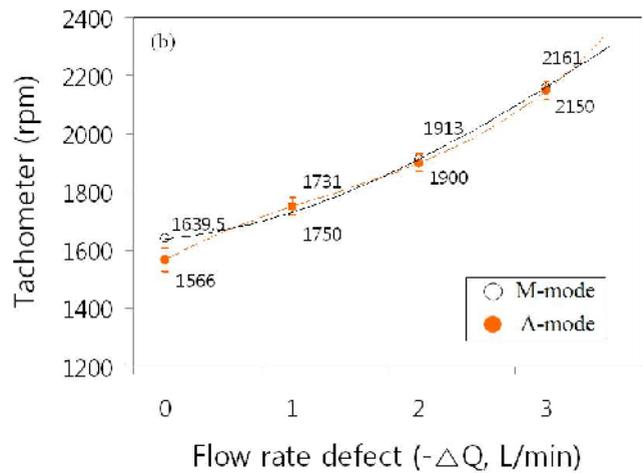
Figure (7): Revolution of driving motor with the variation of flow rate defect : (a) water, (b) corn oil
