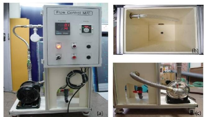
Figure (1): Photographs of constant flow rate control pumping system : (a) display panel and centrifugal pump, (b) circulation reservoir, (c) inlet and outlet piping
