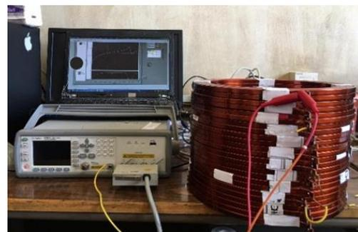
Figure (1): LCR Meter performing DPI magnitude and phase response 20 Hz – 2 MHz of single continuous winding type by the author and supported by the Egyptian National Research Center.
