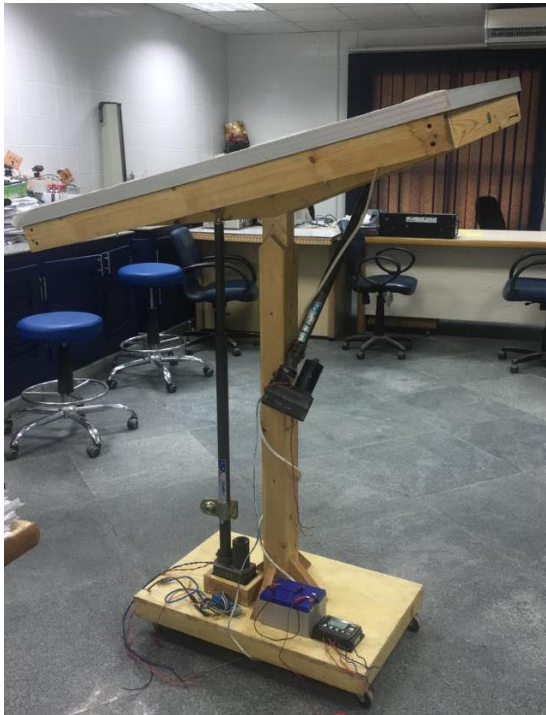
FIGURE (2). A photo of the set-up rig used in measuring the PV I/V, characteristics.
